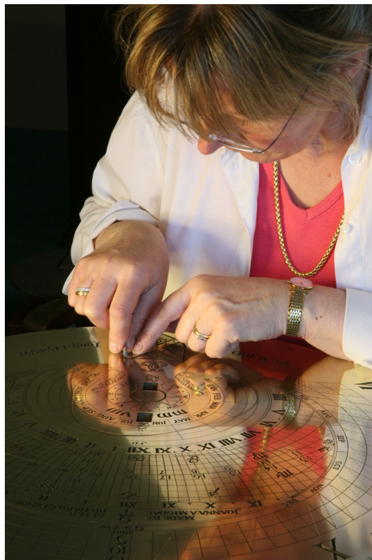
Hand engraving a double horizontal dial.
