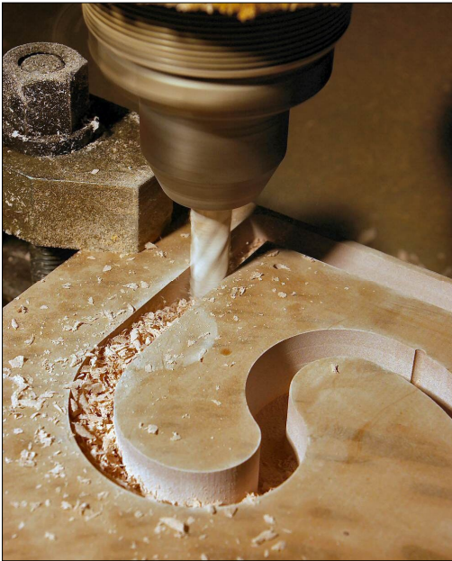
Fig. 6 (top left). Drilling the sundial time line points with a numerically controlled milling machine.
